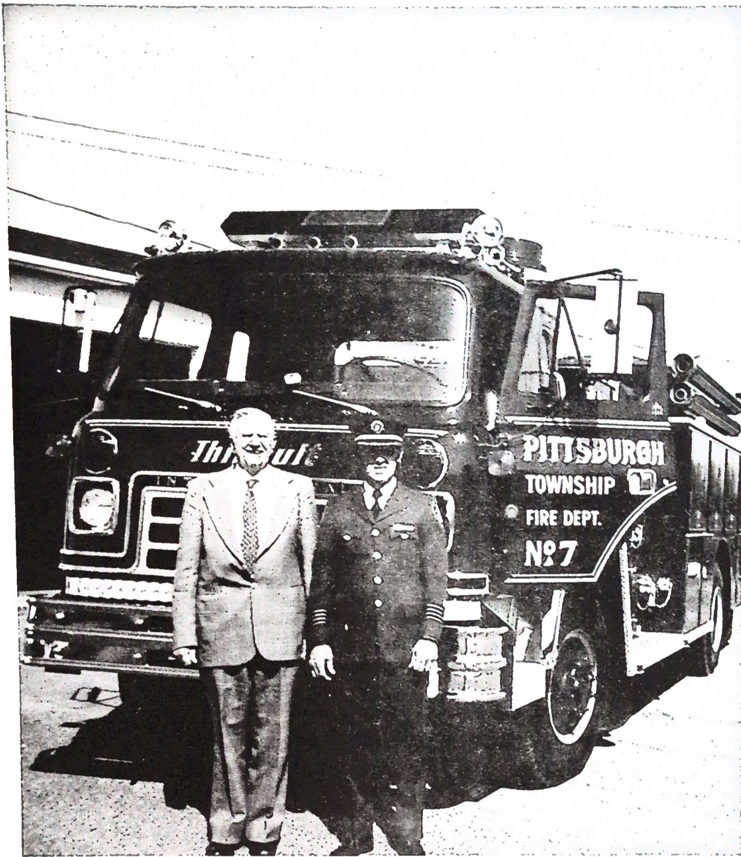
Fire Chief G.W. Bullock and Fire Liason Officer Cameron English with our new triple combination pumper which was delivered in February, 1985. This truck is powered by a Detroit Diesel 6-V71, and built on an International cab chassis. This Unit carries 1000 gals. of water, is prepiped for a deck gun and has a 182" wheel base.
